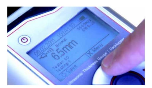
to measure wall thickness, which is key information to calculate the exact inner pipe diameter. It is important to know the exact wall thick-
