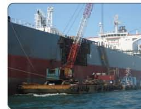
Contact Damage Afloat Repair
