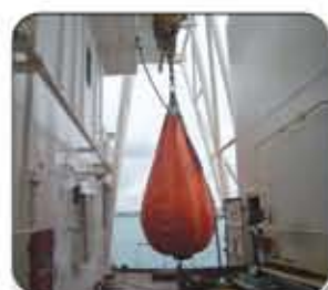
Crane & Davit Load Test
