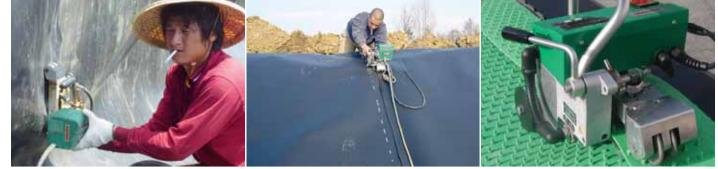
The handy COMET is suitable for a wide range of uses, including vertical welding.
