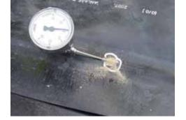
Testing of a welding seam with testing unit and injector needle.
