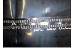
Flawless test welding with the combi-wedge welding machine TWINNY T.
