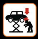
Do not stand under the vehicle on the lift while lift is operating.
