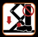
Do not place feet under any moving part of lift while lowering.
