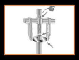
Always check that the pressure screw is properly centered and legshaft secure properly. Lubricate the screw regularly
