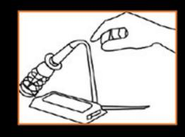
Always rest a hot soldering iron on its stand.
