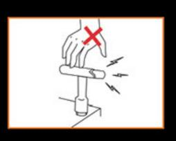
Never use a tool with damaged insulation.
