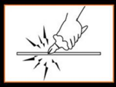
1000V insulated tools must be used when working near live components.
