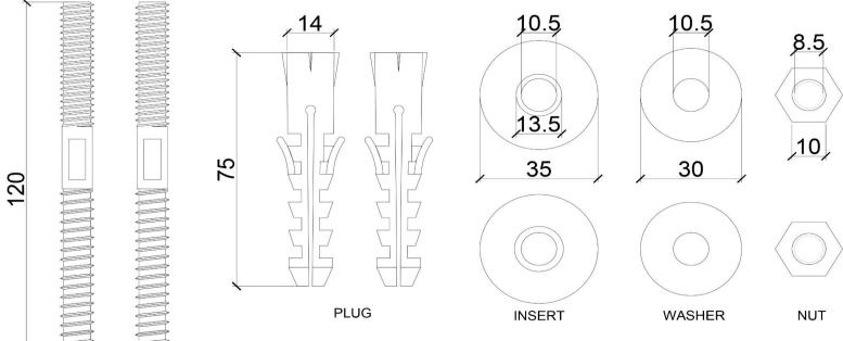
Material: Mild steel with zinc plating finishing
