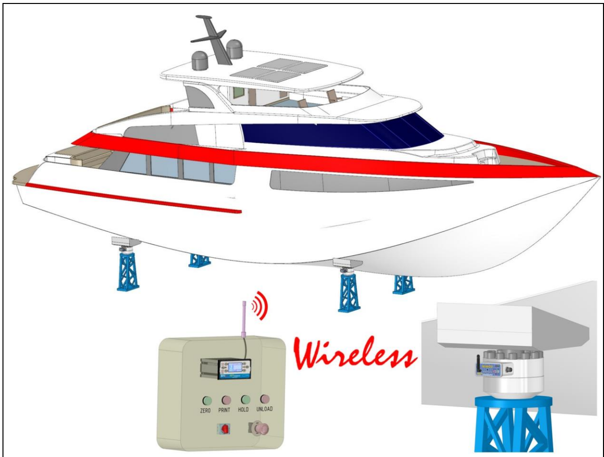
WEIGHT MEASURE: WIMP2Plus + 4 D200 WIMOD load cells Ability to view both the weight measured by each cell that weight TOTAL
