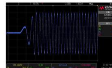
Sudden-load Current wave form, 5.5kW asynchronous motor, 0.5HZ, 60% load
