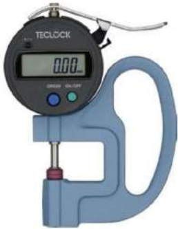
SMD-540S2 Resolution 0.01mm Measuring Range 12mm
