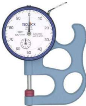
SM-112 Standard type Graduation 0.01mm Measuring Range 10mm
