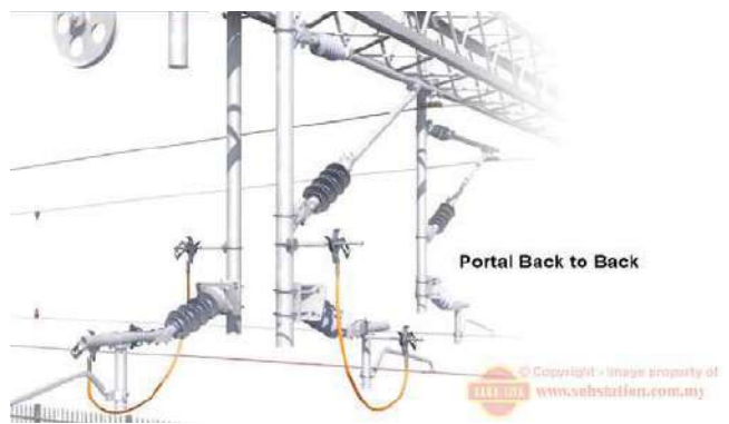
Portal Back to Back using Single Short Rail Earth
