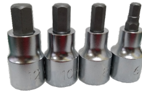
Hex Bit Socket : (From the right) 6mm, 8mm, 10mm, 12mm
