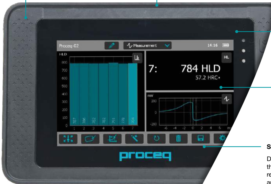
Touchscreen display unit used with the Equotip 550 and 540 impact devices
