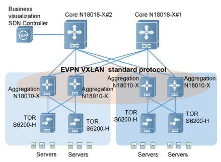
Figure 6: Typical Application of the RG-S6220H Switch Series
