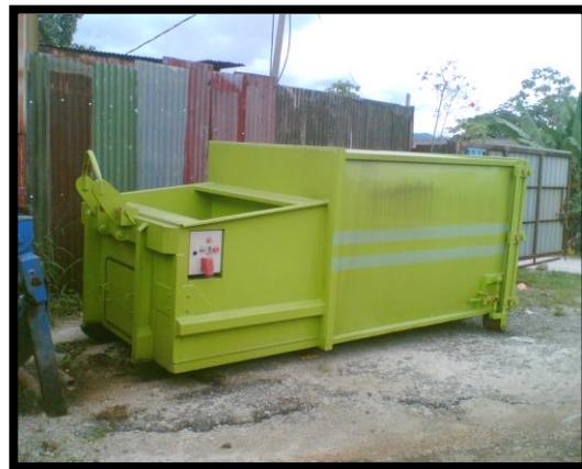
24 CUBIC YARDS PORTABL COMPACTOR (16'L X 5'W X 6'H)
