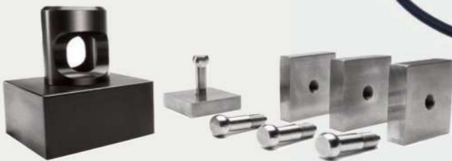
PosiTest AT 50T KIT measures the tensile strength of ceramic tile adhesives.
