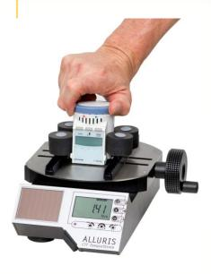
Digital Cap Torque Tester CTT-200 series are particularly suitable as test tools for fast manual torque testing of screw caps, valves, machine components or tools. Objects to be tested (25 - 180 mm diameter) are centrally positioned with retaining bolts and clamped by a contrarotating spindle mounted in the turntable. By manually rotating the test object, the force is transmitted to the torque sensor.
