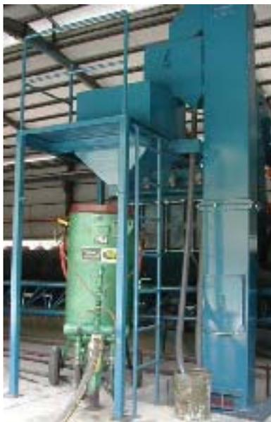
*A Single Double Chamber Blast Pot Silo-Separator-Bucket - Elevator Set-up*
