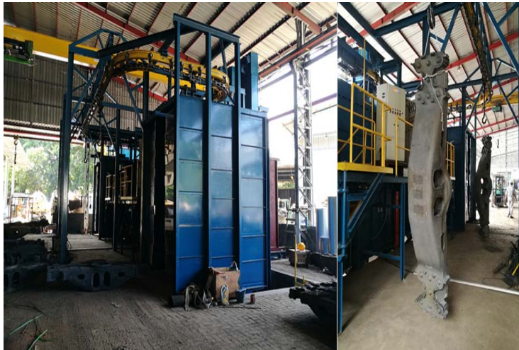
Site Commissioning - Works Pieces are Bogie Bolster and Cast Steel Side Frames at 3 min/pc Through-Put
