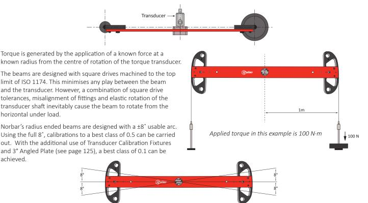
Additionally, the beams are designed to apply load on a vertical plane which cuts through the square drive inside the transducer. This minimises bending moments on the transducer and for safe operation, ensures that the beam will not fall out of the transducer.
