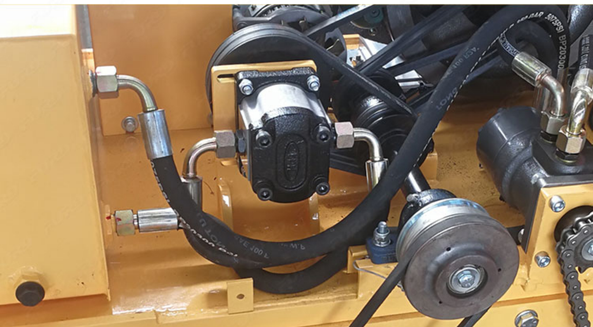
Original imported hydraulic unit, variable speed
