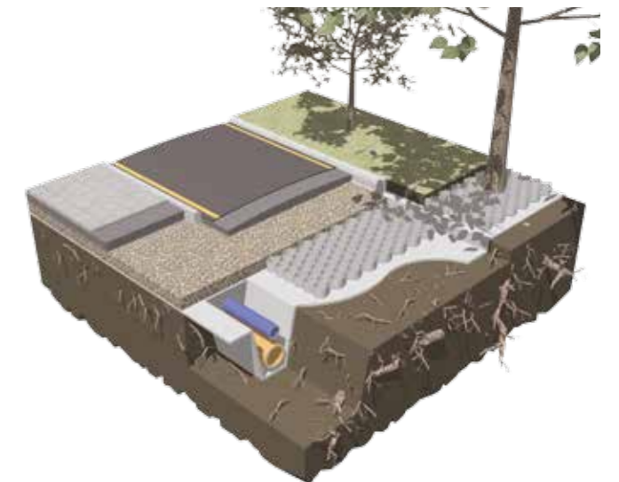
TERRAM Geocell tree-root-protection.
