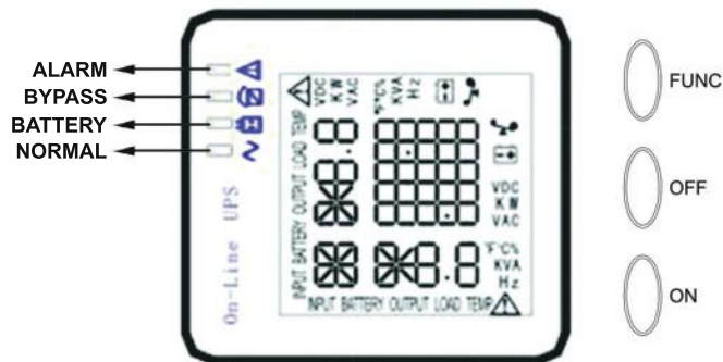
1-3KVA and 10-20KVA LCD display information
