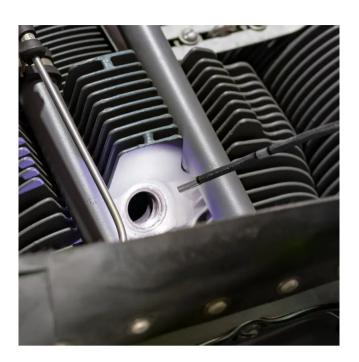
Videoscope for inspecting vehicles, machines, etc.
