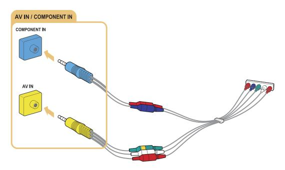
To use component equipment, connect both a component cable (blue) and an AV cable (yellow).
