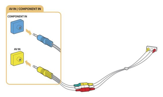
If you want to use AV (composite) equipment, remove the component adapter.
