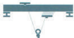
OVERHEAD TRAVELING CRANE
