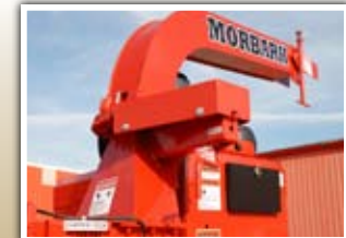
DISCHARGE 360° Manual Crank Swivel Discharge
