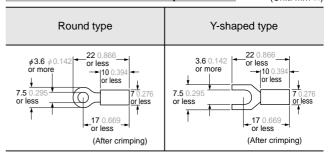
Note: Use crimp terminals with insulating sleeves. Recommended crimp terminal: Nominal size  $1.25 \times 3.5 \ 0.049 \times 0.138$ .
