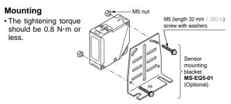
· Care must be taken regarding the sensor mounting direction with respect to the object's direction of movement.
