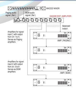
The above illustration is for Uninterrupted Paging setup. In normal setup with single input, use the link switch to form 1 input 8 outputs configuration. Each output from DA2208 can be linked up to 6 power amplifiers.
