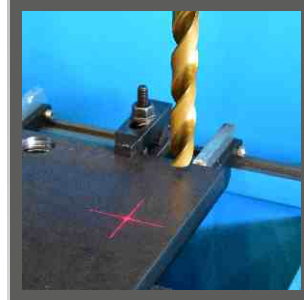
Laser point positioning unit
