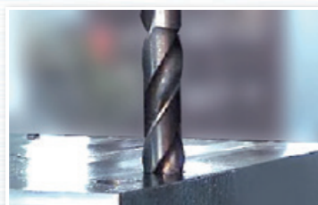
Drilling S45 Ø48mm, 1200rpm, h=100mm 30mm/min, Z axis load 80%, tolerance +0.1mm
