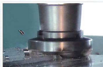
Face cutting S45C Ø150mm, 350rpm, t=8mm 600mm/min, SP load 70% X axis load 28%, RMS 12s
