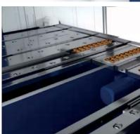
U-gauge with balls in table and suction gauge for smooth handling of the sheet
