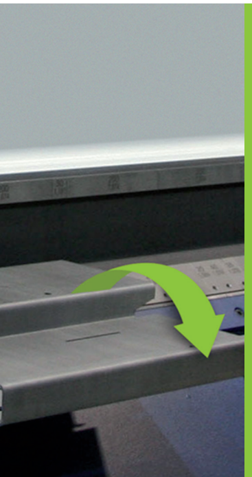
Up-and-Down-function: counter folds without turning upside down the sheet
