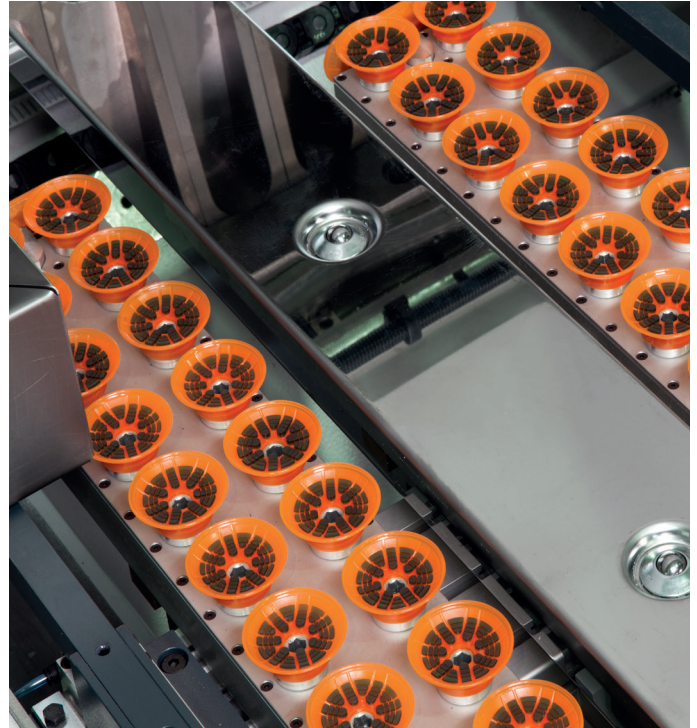
Suction cups in gauge table, controlled via POS 3000.
