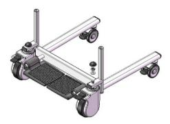
Note: The nut on the top of the 5-inch wheels (not omni-dimensional) must be fitted and fixed into the correct position on the bottom holder.
