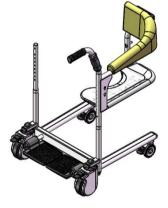
e) Place the handle part into the left shaft, as illustrated on the right:
