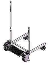
Note: Please press the brakes on the 3-inch wheels before assembly and disassembly.
