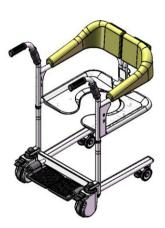
g ) For placing a bedpan, fold the handles on both sides and place the bedpan holder into the hole site, then place the bedpan from the rear, as illustrated on the right:
