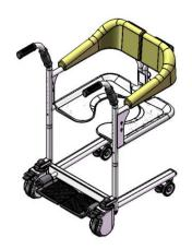
f) Adjust its height by rotating the handle to fit their hole sites into that of the rotatory shafts, then plug into latches. This step is illustrated on the right:
