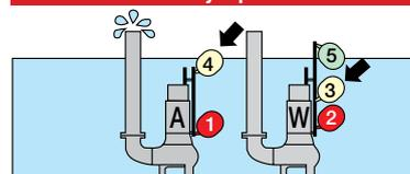
1. Start float 4 of pump A operates to start water discharge. The pump ends primary operation, and stops operating.
