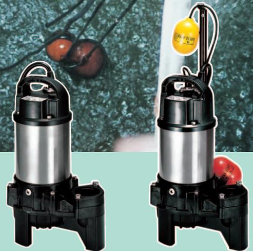
Being made of stainless steel and special resin, the PU-series is not only lightweight but corrosion-resistant as well. Built-in vortex impeller and large passage facilitate pump operations to readily dispose of liquid containing various kinds of foreign matters.
