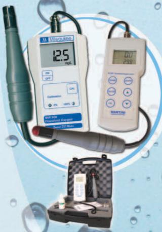
Mi605 is a portable, microprocessor-based, Dissolved Oxygen meter with automatic calibration and temperature compensation (ATC) specifically designed for spot sampling applications. Mi605 is supplied in a hard carrying case with a D.O. probe, spare membranes, calibration solutions, battery and instructions.
