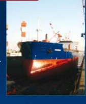
This is the first vessel ever to be coated with polysiloxane technology from Jotun Coatings. The product was chosen as a test bed for gauging the improved performance properties over existing two-pack topcoats. With improved weathering capability and with excellent opacity and gloss retention, Hardtop PS5 provides an owner with a far more versatile coating in the long term than any other two-pack generic topcoat used to date.
