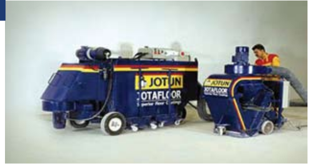
The machine is ducted to a vacuum unit separating dust and reusable steel shot.
