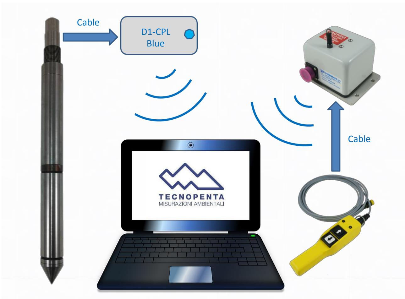
The picture above shows how the data are transmitted. Notice that the data are acquired and stored by the computer via the software **PuntaD**.
