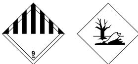
**Marking** : The environmental hazardous / marine pollutant mark is only applicable for packages containing more than 5 litres for liquids and 5 kg for solids.
