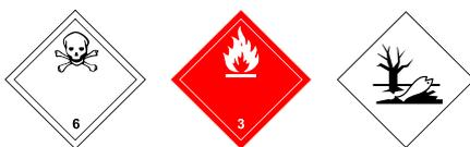
**Marking** : The environmental hazardous / marine pollutant mark is only applicable for packages containing more than 5 litres for liquids and 5 kg for solids.
