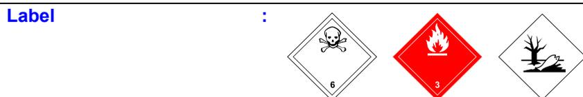
**Marking** : The environmental hazardous / marine pollutant mark is only applicable for packages containing more than 5 litres for liquids and 5 kg for solids.
