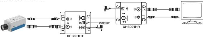
Remark: Please use the attached F connectors for cable connection to avoid any other interference.
