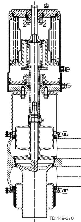
Fig. 1 Details of Unique **PMO Plus**® Mixproof Valve
