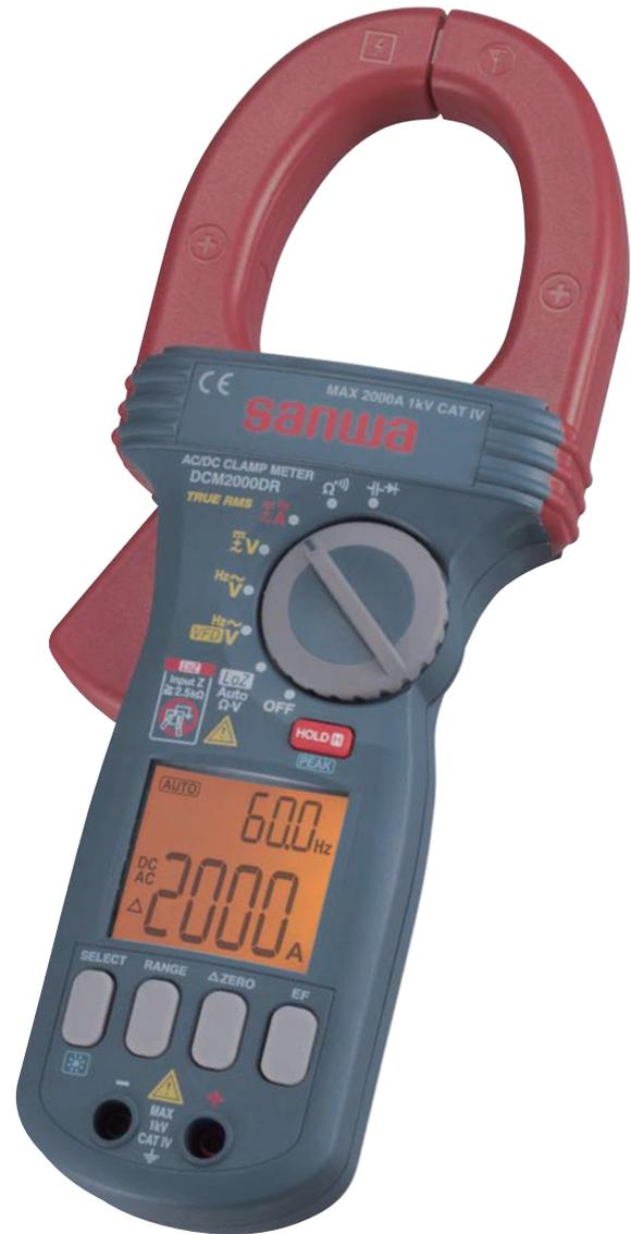
This instrument is an AC/DC clamp meter/digital multimeter of the RMS value response type, designed for measurements in the range specified by IEC 61010-1 CAT. IV 1000 V. It is suitable for current and voltage measurements of lowvoltage circuitry, electric equipment and power supply facilities.
