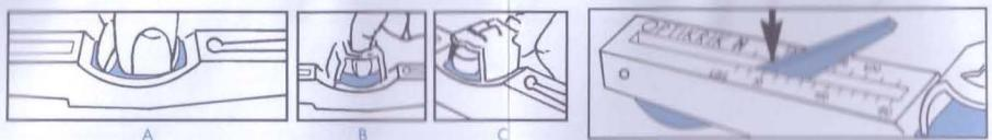
1. Select the gauge appropriate to the belt section and construction being tensioned. See notes below the simplified tensioning table.
