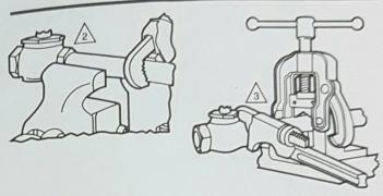
USE PROPERLY REAMED AND CLEANED PIPE AND MODERATE AMOUNT OF DOPE (LEAVE TWO THREADS BARE).
