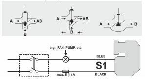
Fig. 13. Application example of auxiliary switch
