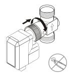
Fig. 3. Mounting the actuator
