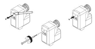
Fig. 9. Adjustment of auxiliary switch S2
