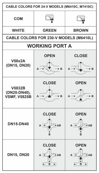
Fig. 5. Cable colors, valve action
