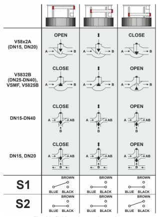
Fig. 11. Cable colors, valve action
