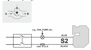
Fig. 12. Application example of auxiliary switch
