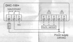
The red wire is "+", which is to connect terminal 4; The black wire is "-", which is to connect terminal 5; The yellow wire is "V", which is to connect terminal 6.
