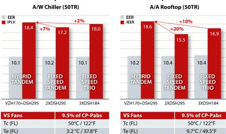
Variable-speed technology improves performance on otherwise poorly modulated systems, with rooftop units and chillers seeing the greatest benefits.
