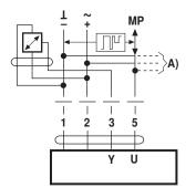
Connection of external switching contact
