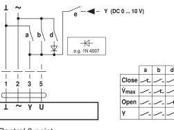
Override control and limiting with DC 24 V with relay contacts
