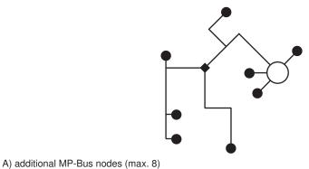
There are no restrictions for the network topology (star, ring, tree or mixed forms are permitted). Supply and communication in one and the same 3-wire cable
