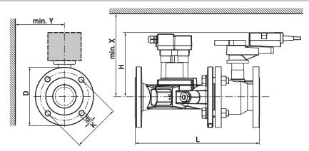
If Y <180 mm, the extension of the hand crank must be demounted as necessary.
