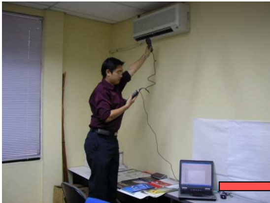
Air-Cond Indoor Unit Air Velocity Measurement (with Vane)
