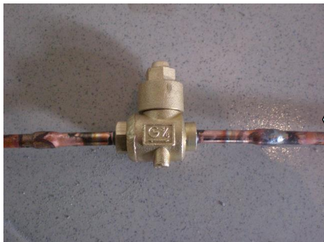
Ball Valve with perfect brazing result
